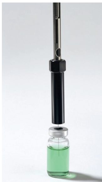
Figure 1: SPME fiber holder with fiber immersed into aqueous sample
